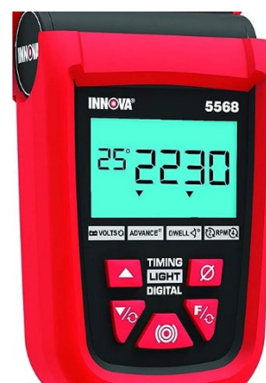
Fig. 1-3. Control panel showing 25° of advance at 2230 RPM.
